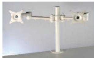
**JFE1261** – White Double FSA Flat Screen Arm. Manually height adjustable. Includes both desk clamp (fits 16-34mm desk thickness) and through desk fixing, (fits 16-55 mm desk thickness). 13kgs max per arm. 30" max screen size.
